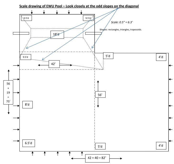
Above is the scale drawing of the EWU Pool. How many sections would you use to divide it up? Notice that only one section has a flat bottom, and that's 18' deep. Next time, we'll look at how to calculate chemical dosages.
