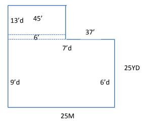
Now we'll calculate each section.  $P_1$ : 75' X 82' = 6150 ft<sup>2</sup>. This is the surface area. To get the volume, we need the average depth: 6' + 9' = 7.5'. The volume is the surface area X the depth = 6150 ft<sup>2</sup> X 7.5' =  $\frac{1}{2}$
